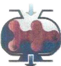
Using a patented development by Aerzener Maschinenfabrik, these pulsations are almost eliminated at source. To achieve this the three-lobe blower has two channels cast into the cylinder wall that control the backstream of gas into the cylinder. This backstream produces sound waves which by interference cancel most of those produced by the blower.
