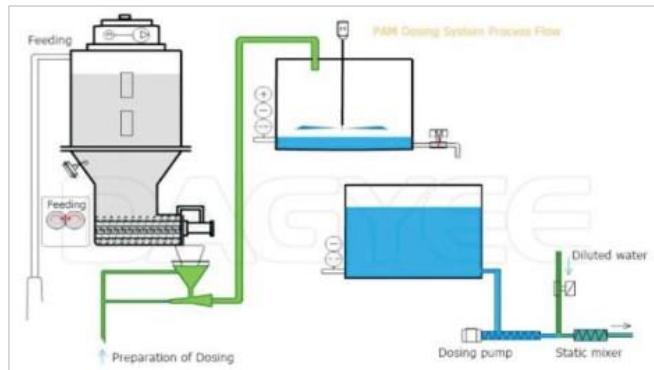
Polymer preparation with three tanks for mixing chemical with water. dosing port at the top for filling chemical and water; the bottom has a sewage outlet for cleaning solution tank. This dosing device used for dosing PAM (polyacrylamide) which can realize integration of PAM powder feeding, dissolving and dosing. The device integrates both automatic and manual operation.
