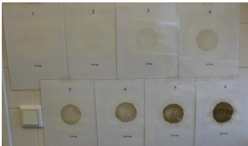
FIG. 3.11 Reference filter papers for membrane integrity assessment ( from the Heenvliet site ).
