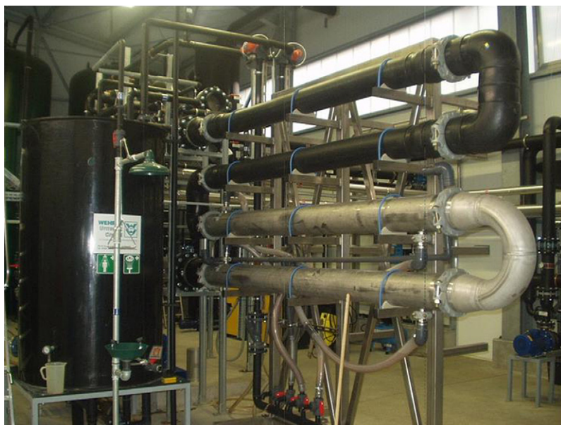
FIG. 2.23 sMBR pilot plant: the total retentate fluid path is four times the length of one horizontal module.
