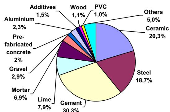
Fig. 2. Contribution of CO<sub>2</sub> emissions associated with the manufacture of the materials needed for the construction of 1 m<sup>2</sup> (gross floor area) [12].
