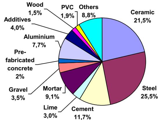
Fig. 1. Contribution of primary energy demand for the manufacture of the materials needed in the construction of 1 m<sup>2</sup> (gross floor area) [12].
