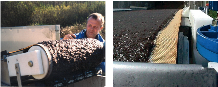
Figure 6.4 Hydrotech belt filter used as secondary water treatment for dewatering the sludge.
