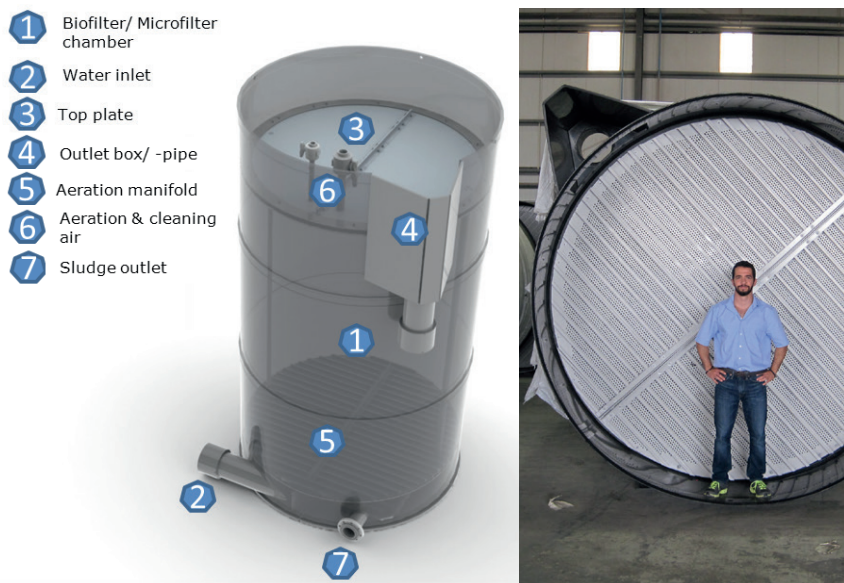
Figure 5.5 Principle drawing of biofilter made of polyethylene (PE) plastic. Normally PE biofilters are placed above ground level fitted with a sludge discharge valve for easy flushing and cleaning. The sludge water is lead to the waste water treatment system outside the aquaculture recirculation system. The picture on the right reveals the size of a large PE biofilter. Source: AKVA group.
