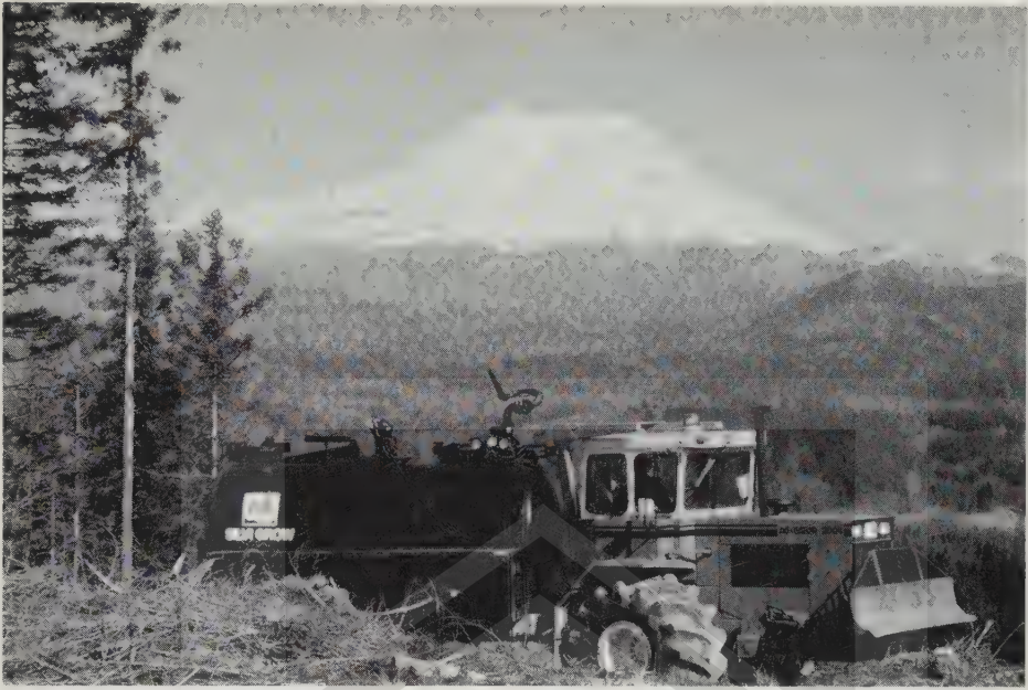
FIGURE 12-47 Forest land sludge application vehicle (from City of Seattle).
