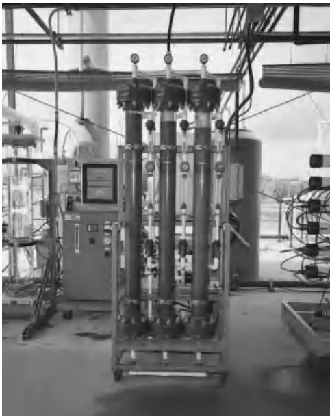
Figure 16-13 Pilot-scale ion exchange column used to verify bench-scale column tests and obtain data on fouling.
