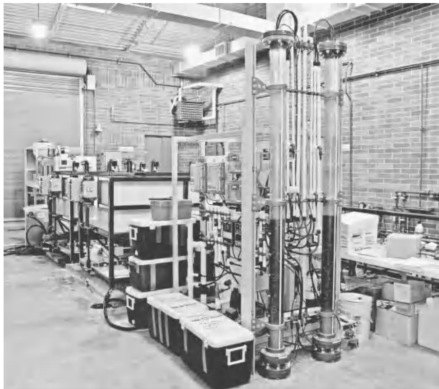
Figure 11-14 Typical rapid granular filter pilot plant and associated facilities. The filters are the tall Plexiglas columns near the front of the photograph.
