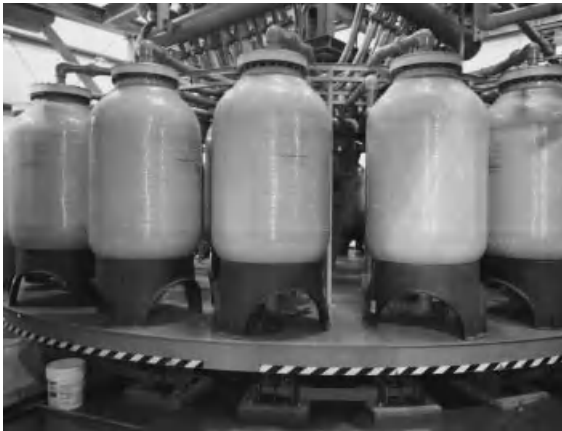
Figure 16-9 Photograph of ion exchange cannisters on rotating platform in Calgon ISEP ion exchange process (see Fig. 16-8).
