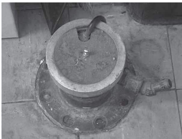
Figure 1.4 Capped, in-floor immersion tank located at Boelter Hall that was used by Loeb and Sourirajan to cast tubular cellulose acetate membranes at UCLA, as viewed in 2008.
