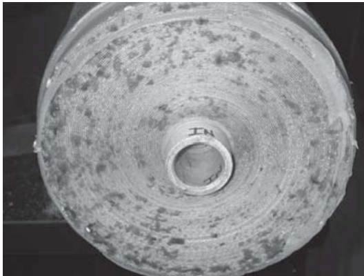
Figure 14.10 Feed end of membrane module showing foulants.
