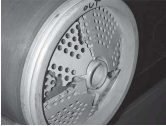
Figure 14.9 Cracked end cap as the concentrate outlet.
