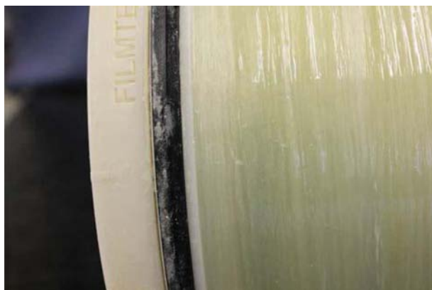
Figure 7.1 Elemental sulfur deposit on brine seal.
