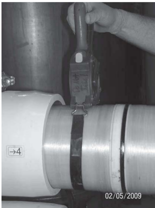
Figure 4.21 Use of strap wrench with iLEC membranes. Courtesy of Crossbow Water Technologies.
