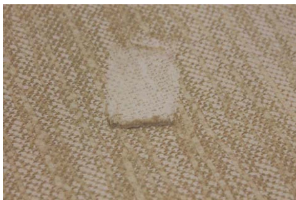
Figure 7.3 Gray deposit of elemental sulfur on the surface of the membrane. Note the incomplete scraping even with manual means.
