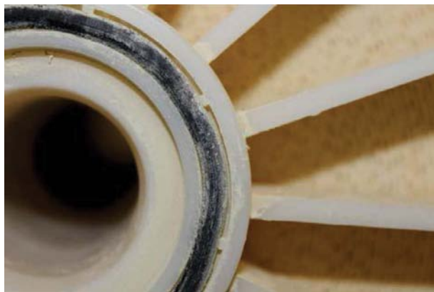
Figure 7.2 Elemental sulfur on iLEC interconnector O-ring seal.
