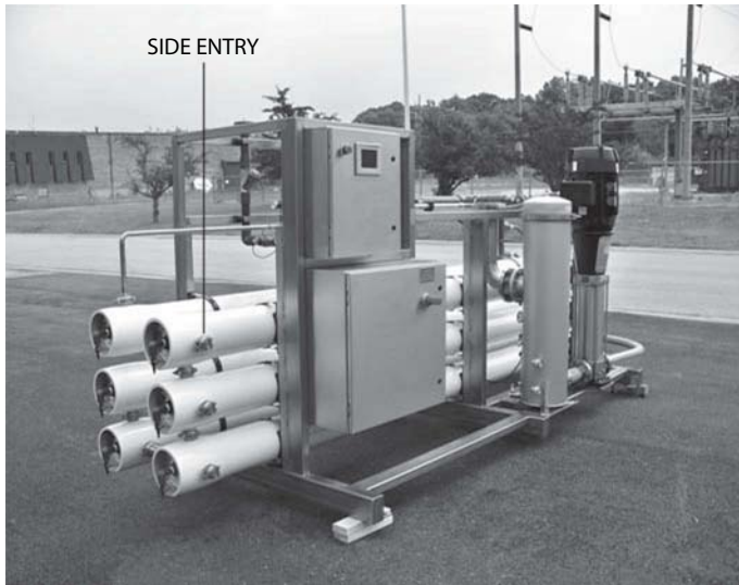
Figure 6.9 Pressure vessel showing side entry of feed water. Courtesy of Nalco-Crossbow Water LLC.
