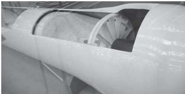
Figure 4.26 Cut-away of a pressure vessel with a spiral-wound modules inside.
