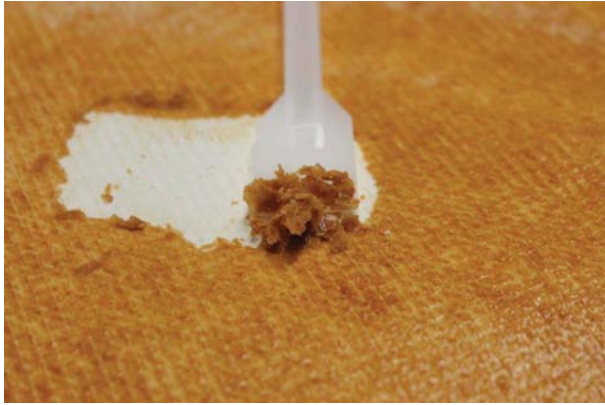
Figure 14.16 Surface of a scaled membrane
